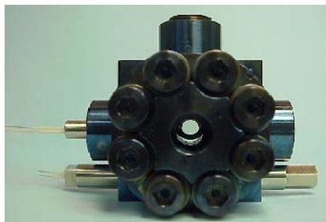
**Fig. 1** Experimental cell for experiments on near critical pure water, in the High Temperature Insert inside the DECLIC CNES facility.
