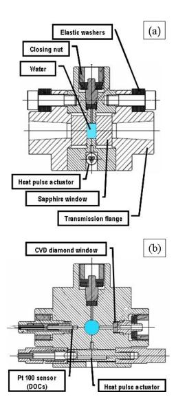
Fig. 2 (a) Cross section of the optical cell showing the optical channel for light transmission observation and de-tails of the mechanical assembly; (b) Cross-section showing the optical channel for 90° light scattering measurements through a CVD diamond window, and the details of the Pt100 temperature sensor (DOCs) and heat pulse actuator.
