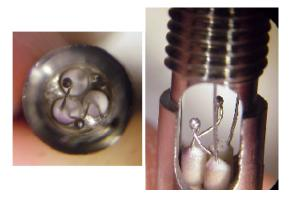
**Fig. 3** Detail of the heat pulse actuator, showing the serial assembly of three Pt100 sensors.
