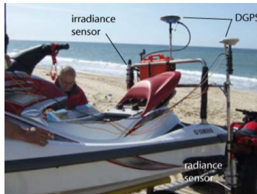
Figure 2. Sensor deployment on board the jet-ski during the hyperspectral field experiment on April 5, 2008
