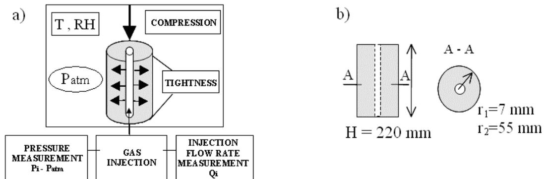
Figure 2: a) Simplified diagram of the experimental device
