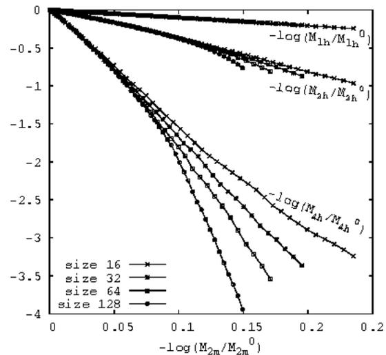
Figure 15: Hydraulic moments vs.  $M_{2m}$  until peak load
