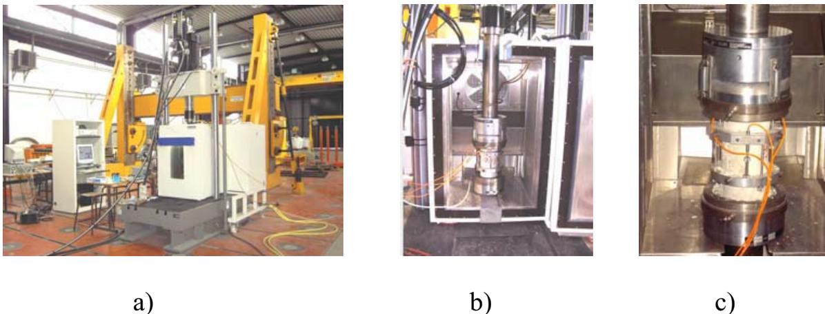
**Figure 3:** Test configuration a) Overall view b) Temperature device c) Mechanical set-up (LVDTs) and permeability cell.
