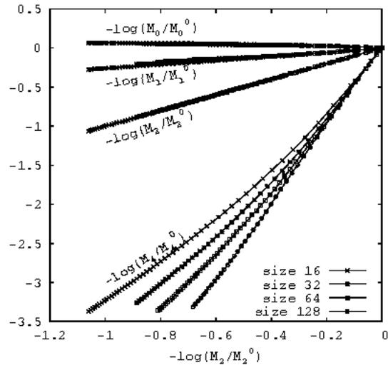
Figure 14: Hydraulic moments vs.  $M_2$  until peak load
