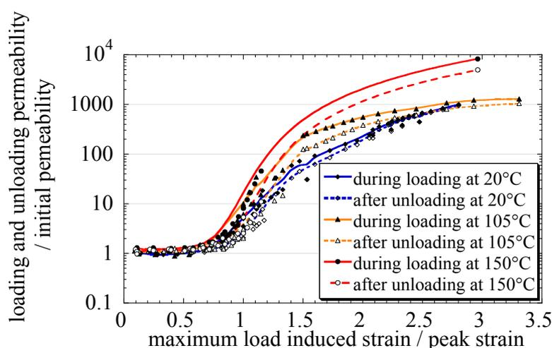
**Figure 11:** Variation of relative intrinsic permeability with maximum applied relative strain for the three tested temperatures. Measurements carried out at temperature, during loading and after unloading
