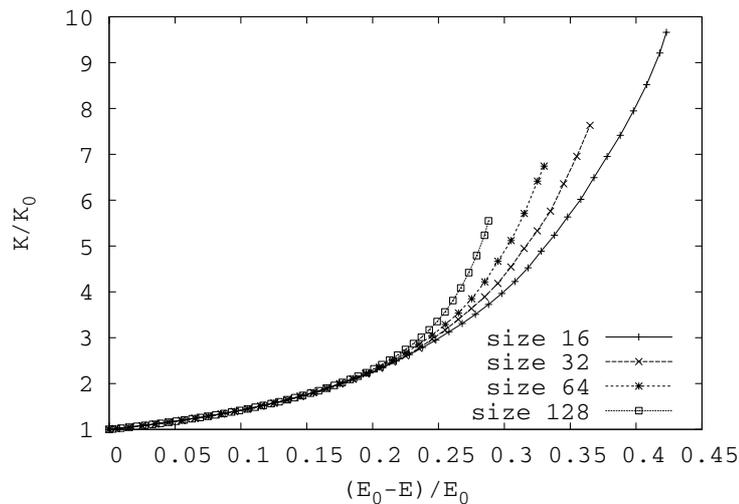
**Figure 17:** Permeability vs. mechanical damage
