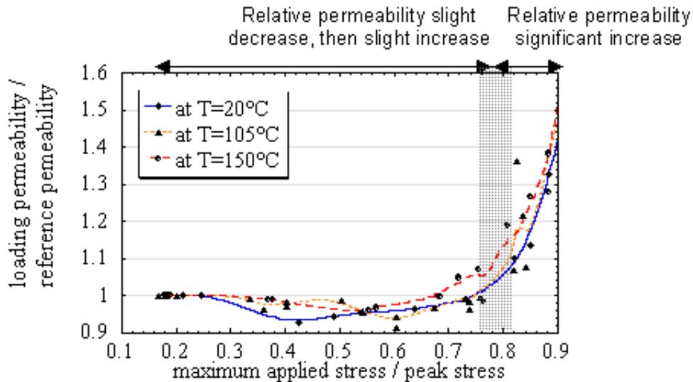
**Figure 8:** Variation of intrinsic permeability values with loading for tested temperatures
