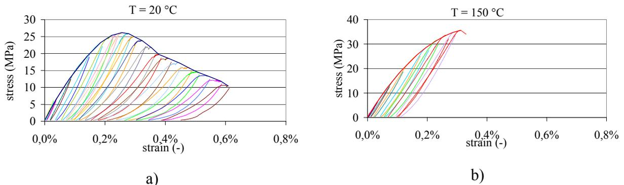
Figure 4: a) Typical stress-strain relation at 20 °C
