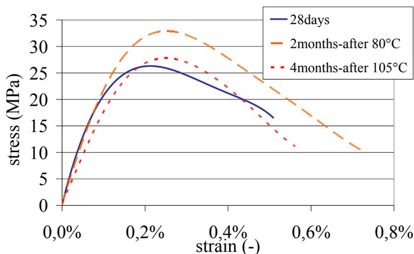
**Figure 1:** Stress-axial strain curves of tested concrete (at ambient temperature)
