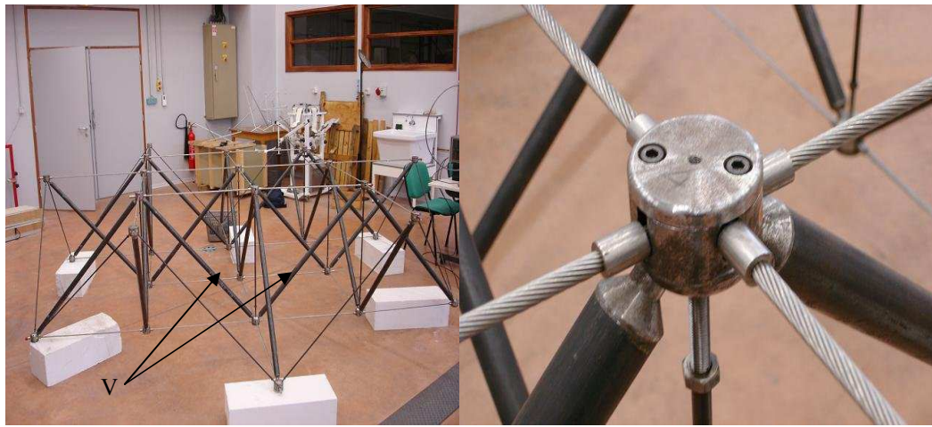
Figure 1. The mini grid: a) general view, b) close up of a node.
