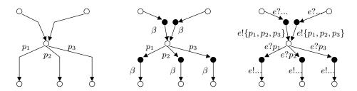
**Fig. 2.** Transformation from atomic BIP components (left) towards atomic components with partial states (middle) and io-machines (right)
