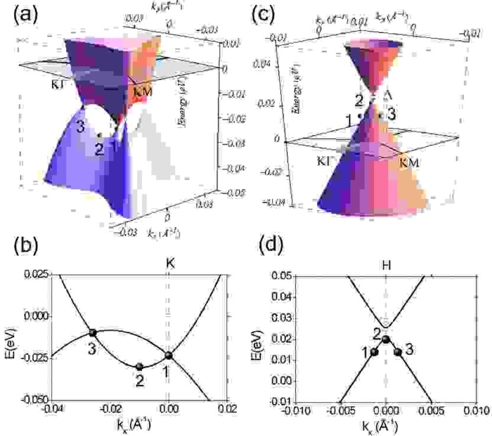
FIG. 7: TB-GW QP band structure around (a,b)  $K$  point, (c,d)  $H$  point. The points 1,2 and 3 denote the dispersion we use to determine electron and hole masses (see Fig. 9). The points 1,2 and 3 span a parabola. In (a,b) the parabola is along the  $KM$  direction with heaviest electron masses and in (c,d) the hole masses are isotropic around  $H$ . Note that the parabolas along 1 – 3 are used for evaluation of the effective electron and hole masses.
