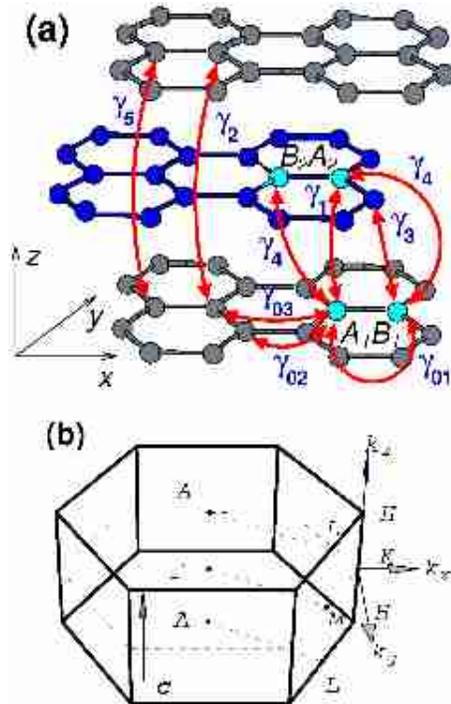
FIG. 1: (a) The graphite unit cell consists of four atoms denoted by  $A_1, B_1, A_2$  and  $B_2$  (light blue). The red arrows denote the interatomic tight-binding hopping matrix elements  $\gamma_0^1, \gamma_0^2, \gamma_0^3, \gamma_1, \dots, \gamma_5$ . The overlap matrix elements  $s_0 - s_3$  (not shown) couple the same atoms as  $\gamma_0^1 - \gamma_0^3$ . (b) The 3D Brillouin zone of graphite with the high symmetry points and the coordinate system used throughout this work.
