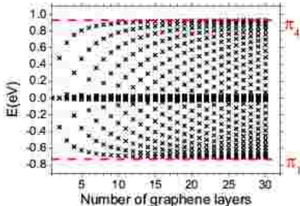
FIG. 13: Evolution of the eigenvalue spectrum for FLG from  $N = 1 \dots 30$  graphene layers calculated by TB-GW at the  $K$  point. The dashed lines labelled by  $\pi_1$  and  $\pi_4$  denote the lower and upper limits of the total bandwidth at  $K$  point in 3D graphite. A pattern that connects the first, second etc. energies of FLG is emerging (see text).
