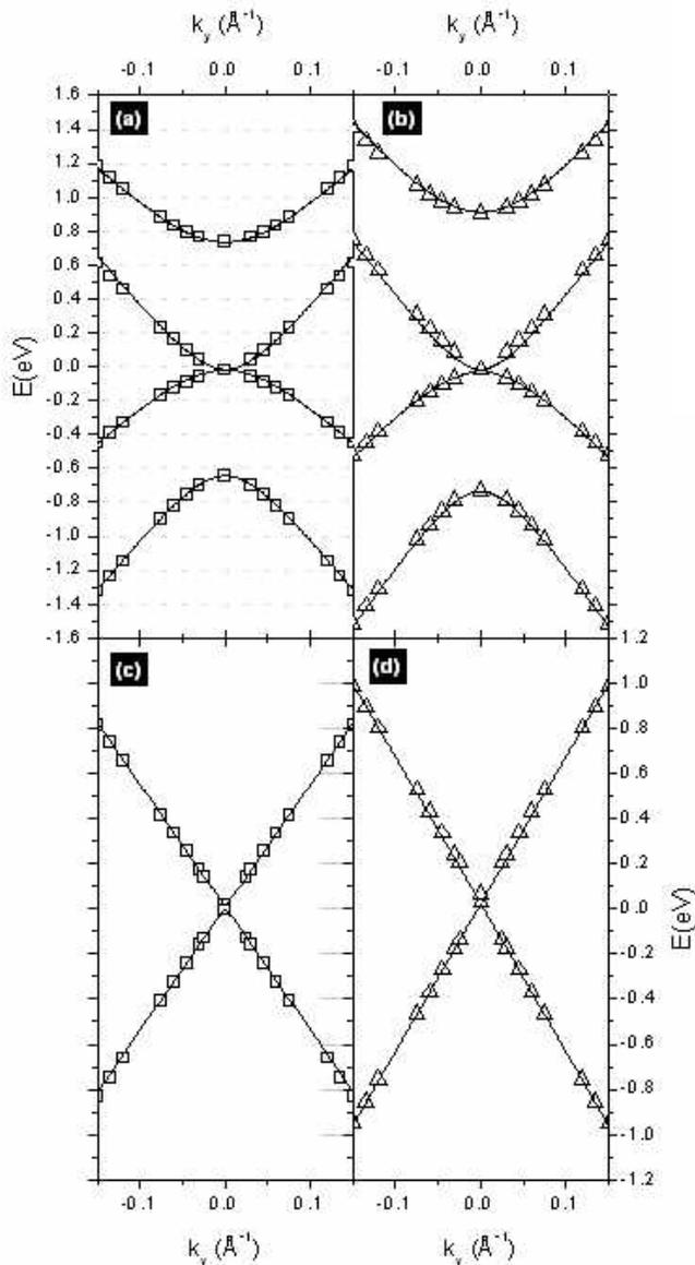
FIG. 3: Upper panel: The TB fits along  $k_y$  direction at  $k_z = 0$  ( $K$  point) for (a) LDA and (b) GW. Lower panel: the  $k_y$  dispersion at  $k_z = 0.47\text{\AA}^{-1}$  ( $H$  point) for (c) LDA and (d) GW.  $\square$  denotes LDA calculations and  $\triangle$  denotes GW calculations that were used for the fitting (taken from Ref. [10]).
