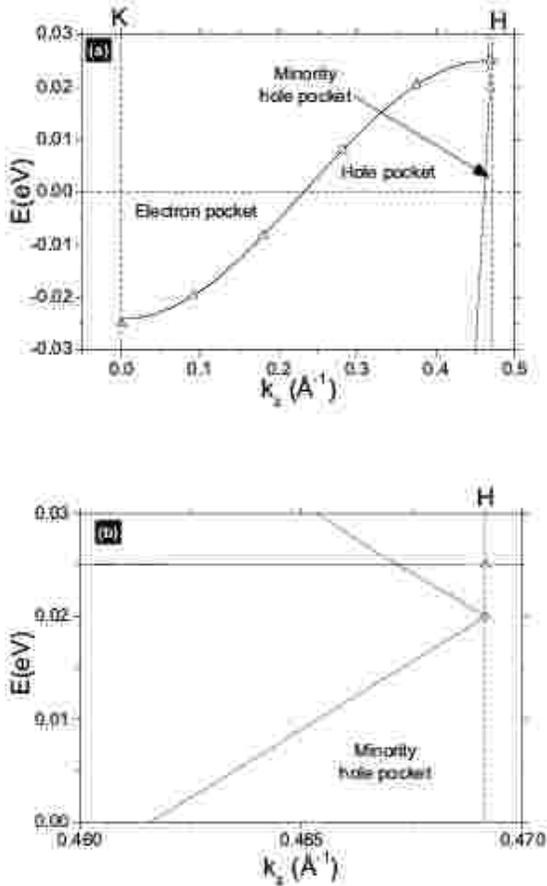
FIG. 6: (a) The weakly dispersive band that is responsible for the formation of electron and hole pockets.  $\Delta$  denotes GW calculations (with the impurity doping level adjusted to reproduce the experimental gap at  $H$  point) and the line the TB-GW fits. (b) shows a magnification of the minority hole pocket that is caused by the steeply dispersive band close to  $H$ .
