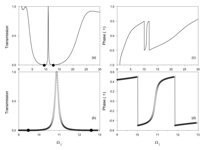
FIG. 2. (a) The same as in Fig. 1(c) but the lengths of the resonators are taken such that  $d_1=0.46d_2$  and  $d_3=0.54d_2$  and N=N'=1. Solid circles on the abscissa indicate the positions of the transmission zeros induced by the dangling resonators on both sides of the resonance. (c) The same as in (a) but for the variation of the phase. (b) and (d) give the approximate results (open circles) around the resonance.
