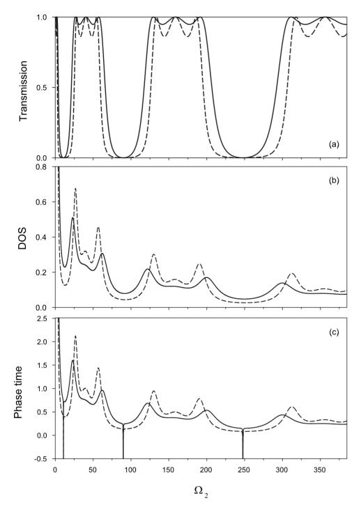
FIG. 6. (a) Transmission coefficient vs the reduced frequency  $\Omega_2$  for the structures depicted in Fig. 1(c) (solid line) and Fig. 1(e) (dashed line). (b) The same as in (a) but for the variation of the density of states (in units of  $d_2^2/2D'$ ). (c) The same as in (b) but for the variation of the phase time (in units of  $d_2^2/2D'$ ). The parameters are  $d_1=d_3=0.5d_2$  and  $\tilde{H}=1$ .
