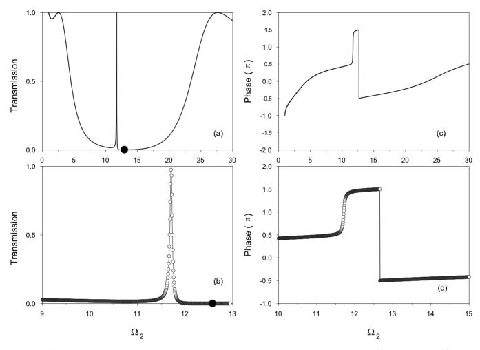
FIG. 3. (a) The same as in Fig. 2(a) but the resonators are taken to be of identical lengths  $d_1 = d_3 = 0.46d_2$ , (c) The same as in (a) but for the variation of the phase. (b) and (d) give the approximate results (open circles) around the resonance.
