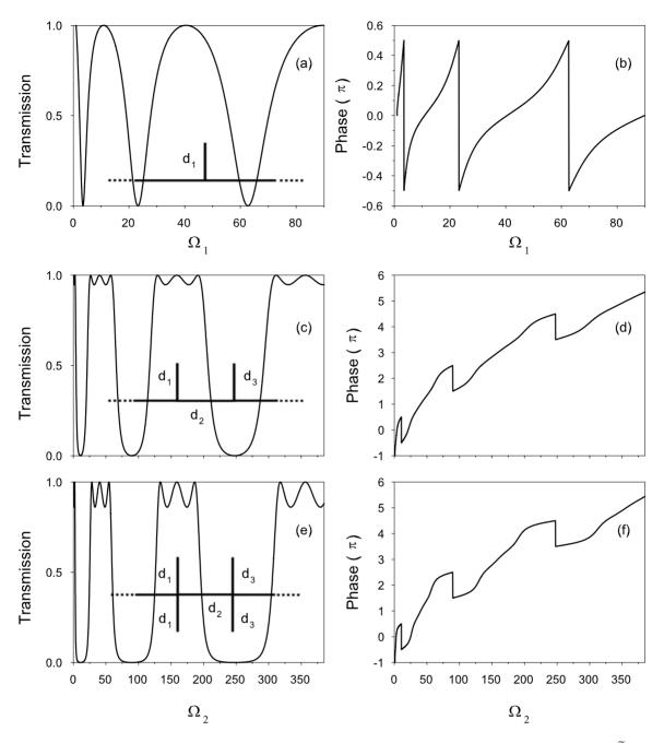
FIG. 1. (a) Transmission coefficient vs the reduced frequency  $\Omega_1$  for the structure depicted in the inset. For convenience  $\tilde{H}'$  is considered to be 1. (c) Transmission coefficient vs the reduced frequency  $\Omega_2$  for the structure depicted in the inset with  $d_1=d_3=0.5d_2$  and N=N'=1. (e) The same as in (c) but for the structure depicted in the inset of (e) (N=N'=2). (b), (d), and (f) are, respectively, the same as (a), (c), and (e) but for the variation of the phase.
