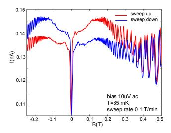
FIG. 1: Current through a pair of ohmic contacts at T=65mK as a function of magnetic field at fixed ac bias of  $10\mu$ V and B-sweep rate 0.1T/min. The red trace correspond to B-field up-sweeps and the blue trace to a down-sweep. As the B-field approaches a value around 0.5 T, the hysteresis disappears.
