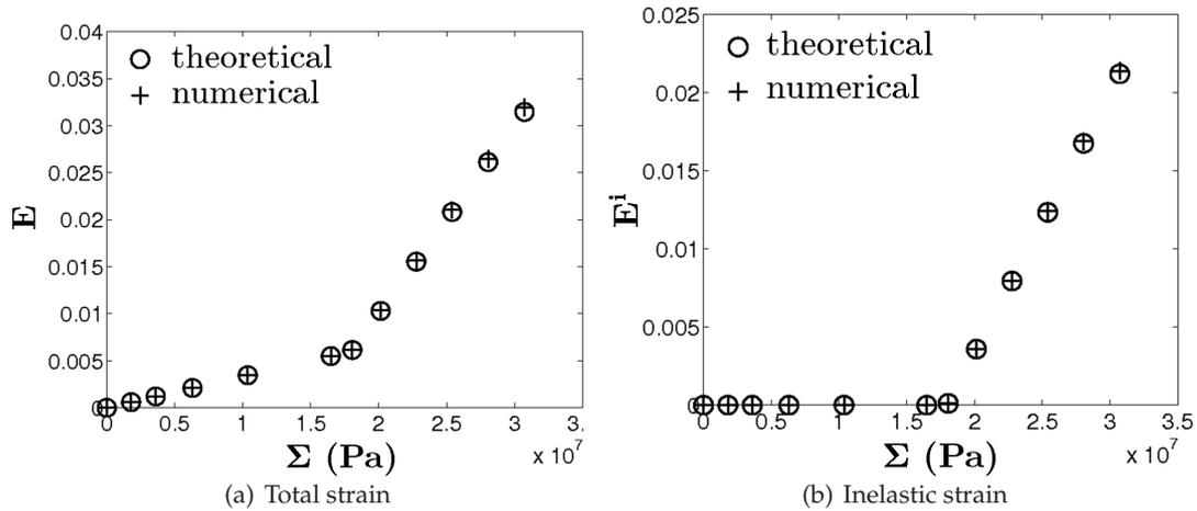
Fig. 4 Stress-strain response of the elasto-plastic composite structure.
