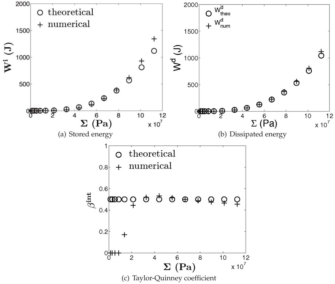
Fig. 9 Energetic response of the frictional composite structure.
