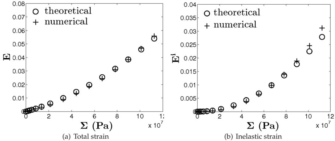
Fig. 8 Stress-strain response of the frictional composite structure.
