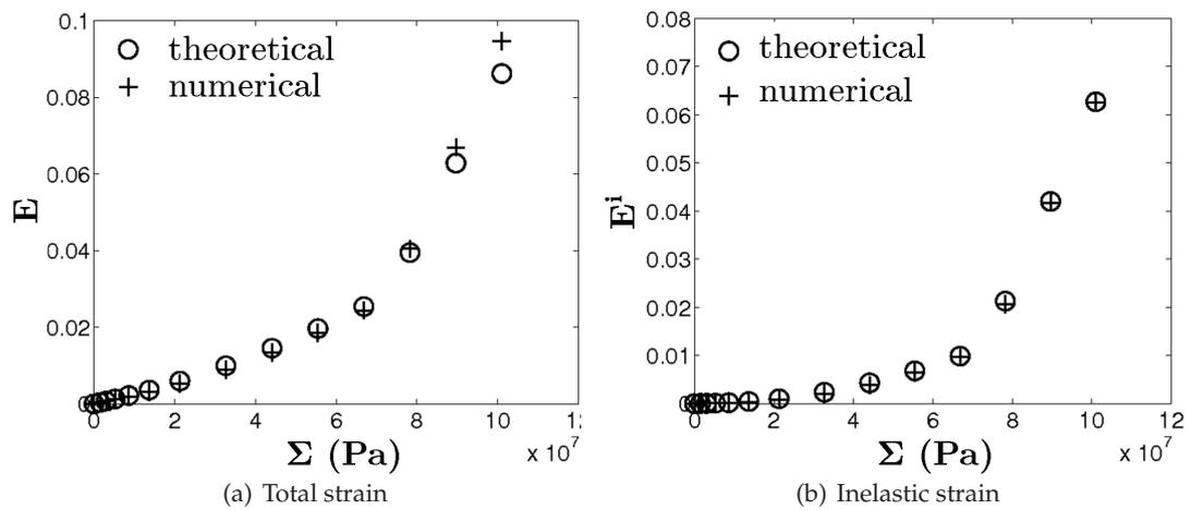
Fig. 11 Stress-strain response of the frictional-plastic composite structure.
