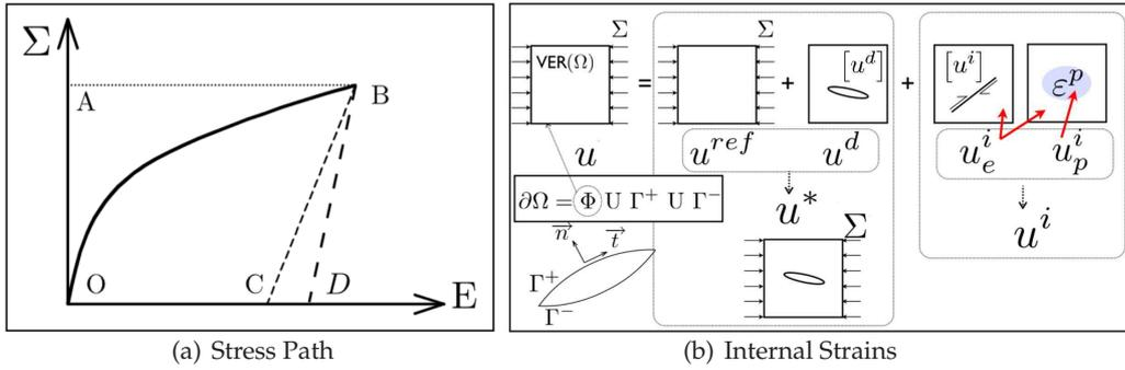
Fig. 2 Stress paths and corresponding displacement decompositions.
