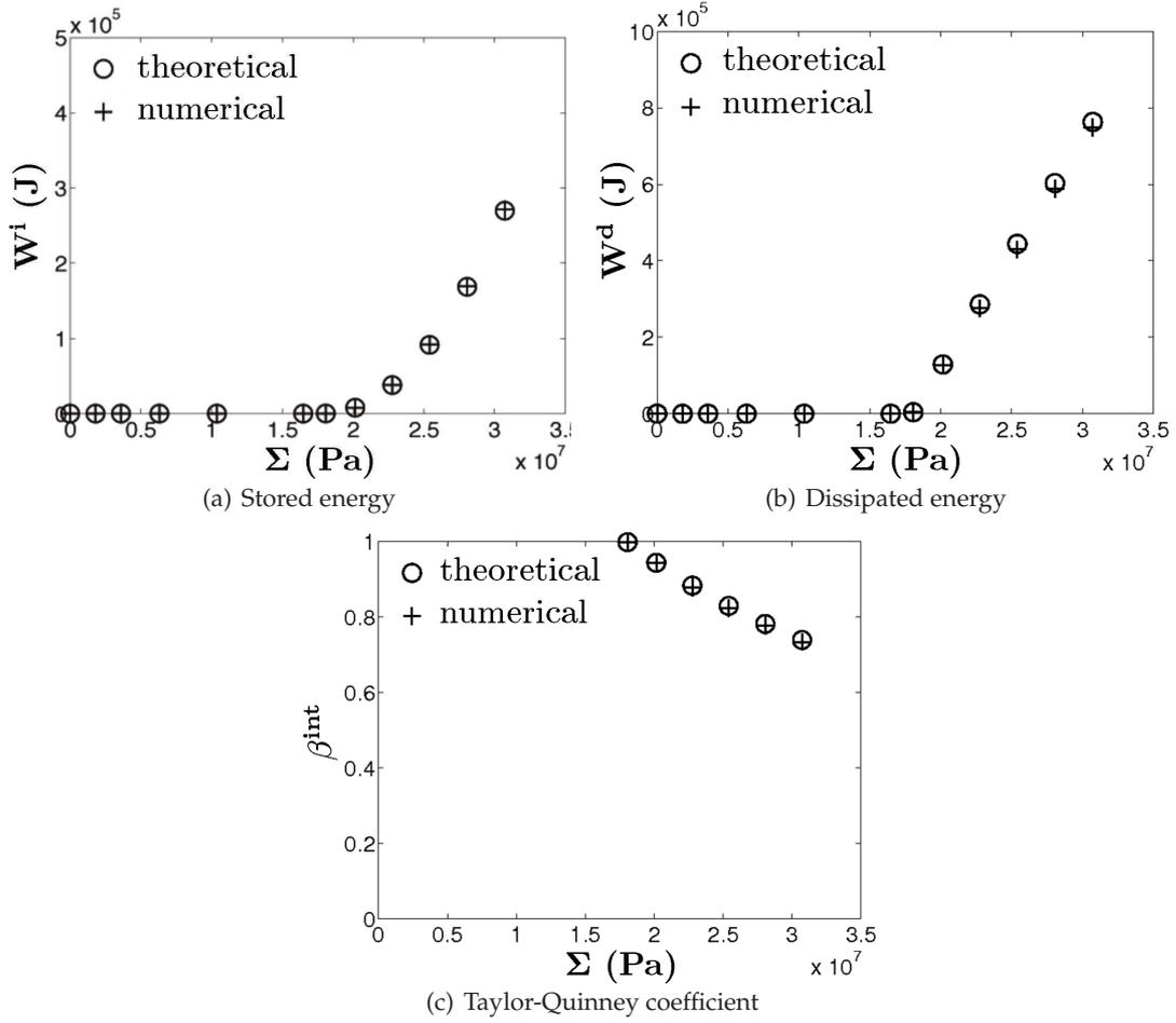
Fig. 5 Energetic response of the elasto-plastic composite structure.
