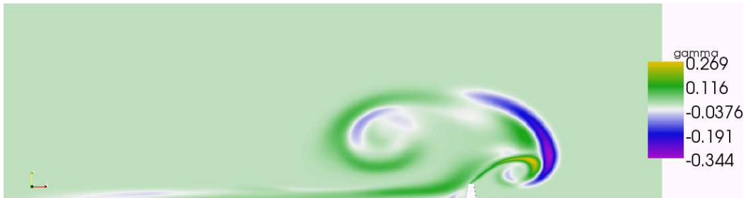
Figure 11. Difference of the volume fraction distributions computed according to the standard and new models at t = 60 s. The color scale ranges from -0.344 to the maximum value 0.269.
