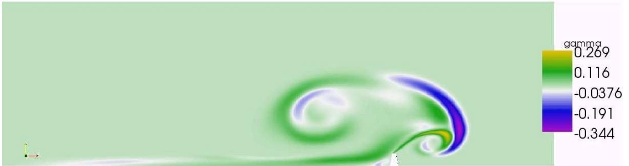
FIGURE 11. Difference of the volume fraction distributions computed according to the standard and new models at t = 60 s. The color scale ranges from -0.344 to the maximum value 0.269.
