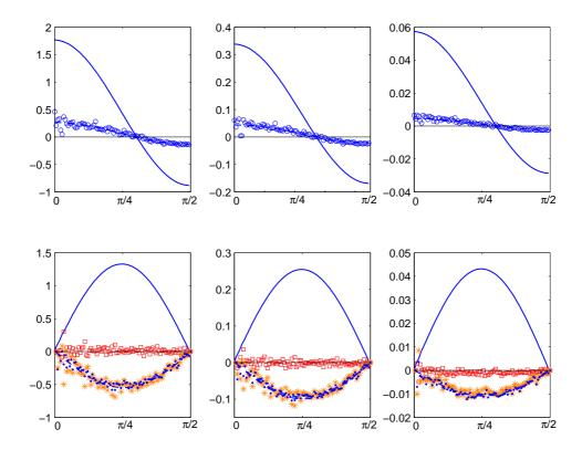
Figure 5: Normal (first row) and tangential (second row) contact displacements for sample A, averaged over equally oriented contacts, at p=10KPa (left),  $p=10^3KPa$  (center) and  $p=10^5KPa$ . The results are in diameter units, multiplied by  $10^4$ . Solid lines indicate the average strain contribution; symbols:  $\bullet = \langle \tilde{w} \rangle$ ;  $*= \langle \tilde{w}^{\omega} \rangle$ ;  $\square = \langle \tilde{w}^{u} \rangle$ .
