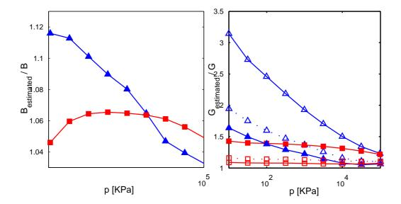
Figure 4: Ratio of estimated to measured bulk (left) and shear (right) modulus for sample  $A(\Box)$  and  $C(\triangle)$ . Filled symbols indicate the results of the average strain assumption; empty symbols indicate the estimate of the shear modulus in the 1FP (dashed line) and the FP approach (solid line).
