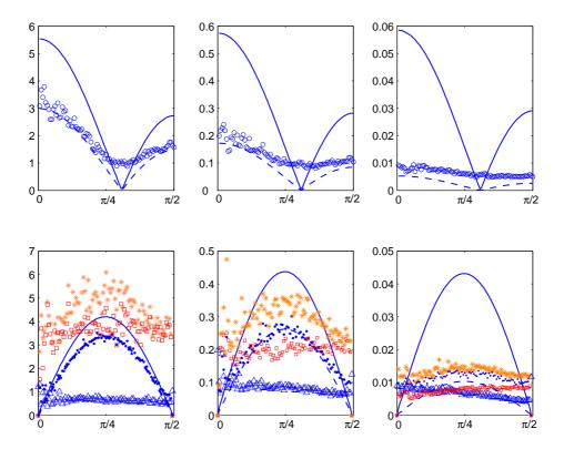
Figure 7: Modulus of normal (first row) and tangential (second row) contact displacements averaged over equally oriented contacts and multiplied by 10<sup>4</sup>. Same symbols as in Figure 5.
