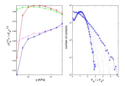
Figure 3: Left-hand side: evolution of the quantity  $\langle F^{1/3} \rangle / \langle F \rangle^{1/3}$  for samples A( $\square$ ), B( $\diamondsuit$ ), C( $\triangle$ ) and D( $\bigcirc$ ). Right-hand side: evolution of the normal contact force distribution for sample C; the dashed and solid line repersent, in turn, the distribution at p=10 and  $10^5 KPa$ ; dotted lines are used at intermediate pressures.
