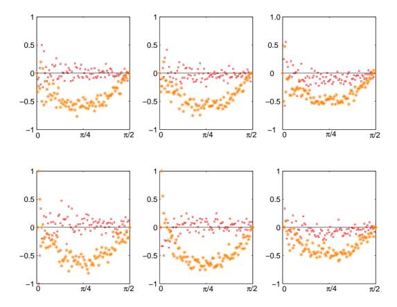
Figure 8: Sign of  $\tilde{w}^u(\Box)$  and  $(\tilde{w}^\omega)(*)$  over equally oriented contacts for sample A(first row) and C (second row), at pressure p = 10(left),  $10^3(\text{center})$  and  $10^5 KPa(\text{right})$ . A positive (negative) value means the dominance of the positive (negative) sign; the numerical value gives the fraction of contacts that sign prevails by.
