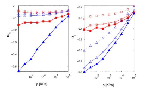
Figure 10: Estimated and measured value of  $\alpha_N$  and  $\alpha_T$  for sample A( $\square$ ) and C( $\triangle$ ). Filled symbols: measured values; empty symbols and dotted line: PF estimate; empty symbols and solid line: 1FP estimate.
