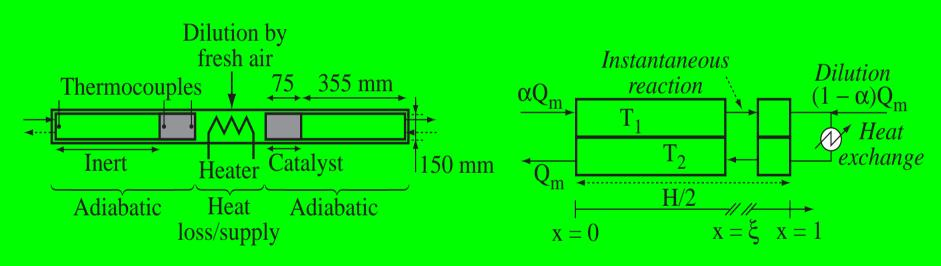
Left: main geometrical characteristics of the RFR. Right: the countercurrent model.
