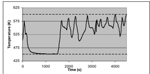
Figure 5: Hot spot temperature (MPC).
