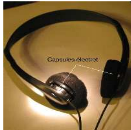
Fig. 15. The “phonocasque” used for the binaural recordings: standard headphones where microphone capsules have been inserted.
