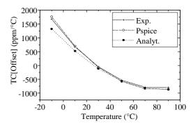
Fig. 3 : Offset temperature coefficient of frequency output.
