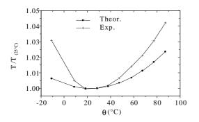
Fig. 2 : Comparison between theoretical and experimental data on relative period variations with temperature.
