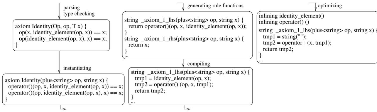
Figure 1. The procedure to compile and optimize axioms
