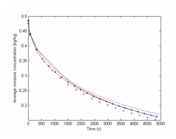
Fig. 2: Reference trajectory tracking: reference curve (•••) for the drying process output: with open loop control while  $u=u_0=[49.5^{\circ}C\ 10.0\%]$  (x) and  $u=u_0=[45.0^{\circ}C\ 20.0\%]$  (---), with the MISO PID (--) and with the MISO MPC (--) with a 5 point horizon prediction, each case with uncertainties: 1.68% error on the initial moisture concentration and 10.0% error on the diffusion coefficient.
