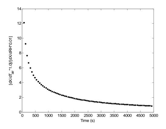
Fig. 5: The ratio between the sensitivities of the air temperature and mean relative humidity with respect to an air temperature input of  $1.0^{\circ}$ C and with respect to a relative humidity input of 1.0%, measured for the drying process at  $49.5^{\circ}$ C and 10.0%.
