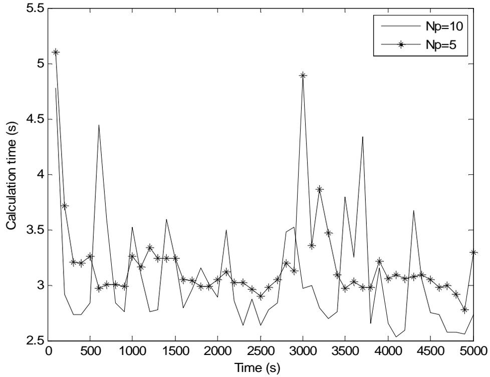
*Fig. 7: Time needed by the whole program to compute the control action by the MPC, evaluated for prediction horizons of 5 (—) and 10 (—\*—) points, each case with uncertainties: 1.68% error on the initial moisture concentration and 10.0% error on the diffusion coefficient.*
