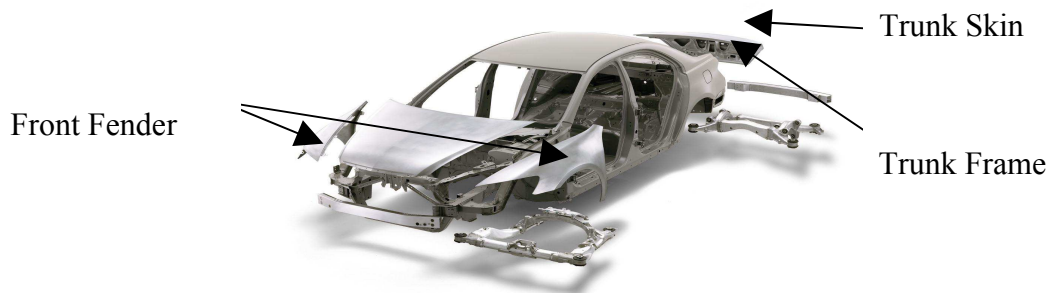
Figure 1 : Aluminum closure panels produced by blow forming
