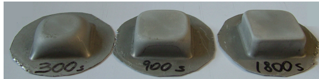
Figure 5. Constant pressure test with 0.7 MPa: formed specimens at three different forming time values (starting from the left 300s, 900s and 1800s).
