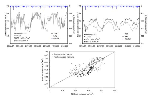
Fig. 2. Surface soil moisture (top left) and root-zone soil moisture (top right) and drawn together (bottom) measured by TDR and obtained by ERS scatterometer from June 1997 to November 2000.
