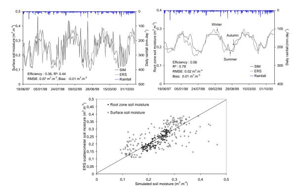
**Fig. 4.** Comparison of surface and root-zone soil moisture  $(m^3 m^{-3})$  for ERS scatterometer data (5 cm and 1 m depth, respectively) and simulation (1 cm and 1.5 m depth, respectively), from June 1997 to November 2000.
