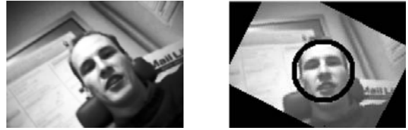
Fig. 8: Face detection after geometrical correction. -On original frame (left) the face detector fails to detect the face, while on the rotated image (right) it detects the face.
