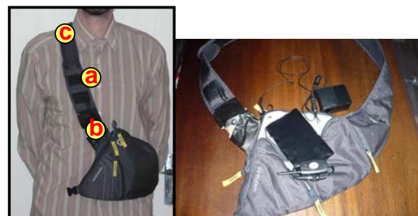
Fig 3. Illustration of the current prototype, with considered camera position (a,b,c). The system is composed of a strap bag which holds a battery, a camera, a microphone, and a wireless transmitter.
