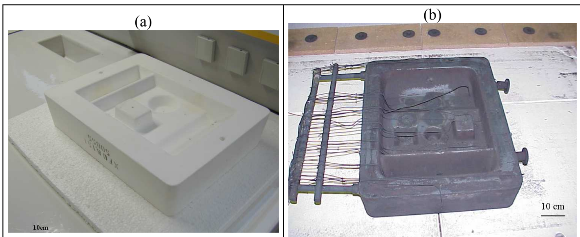
Figure1: a: Silica based ceramic die; b: cast steel die
