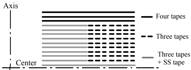
Fig. 3. Conductor distribution within half of the coil.
