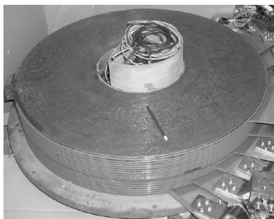
Fig. 5. The pancake magnet under assembling.
