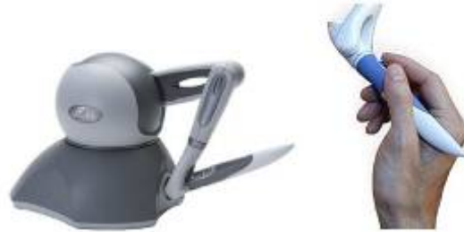
Figure 2: Using the Omni Phantom for the manipulation of the virtual US probe
