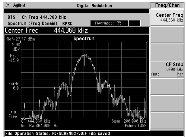
Fig 13 : Spectrum with a simple R ,C filter
