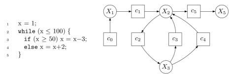
Formally, the set of variables of  $\mathcal{E}$  is  $\{X_1, X_2, X_3, X_5\}$ , representing the value of the variable x at program points 1, 2, 3 and 5. The set of commands of  $\mathcal{E}$  is  $\{c_0, c_1, c_2, c_3, c_4, c_5\}$ , with:
