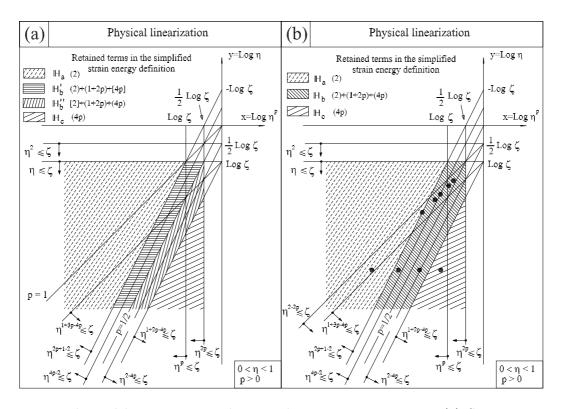
Fig. 9. Physical linearization and Navier kinematic assumptions. (a) Strain rotation domains. (b) The strain-rotation domains, where  $\mathbb{H}'_b$  and  $\mathbb{H}''_b$  are merged. The "strain-rotation points" represent the deformed configurations of the structures of the examples discussed in Section 8.2.
