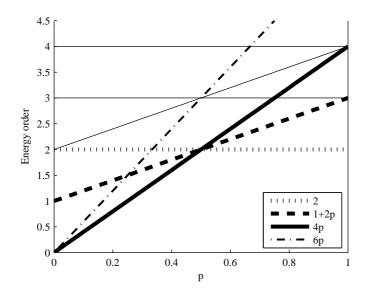
Fig. 8. Navier kinematic assumptions and orders of the strain energy terms. The dominant terms (2, 1 + 2p and 4p) are highlighted. The line corresponding to the order 6p represents the most important energy term associated with the non-linear constitutive law (8). Note that the terms of order 3 + p, 2 + p and 1 + 3p no longer appear (compare with Figure 2).
