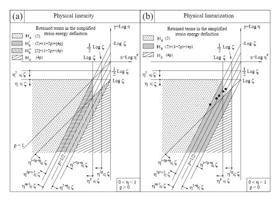
Fig. 3. (a) Strain-rotation domains for a physically linear material. (b) Strain-rotation domains under the assumption of physical linearization. The sets  $\mathbb{H}'_b$  and  $\mathbb{H}''_b$  are merged into the set  $\mathbb{H}_b$ . The "strain-rotation points" represent the deformed configurations of the structure of the numerical example discussed in Section 5.3. In both Figures (a) and (b), the dominant terms of the strain energy are indicated.
