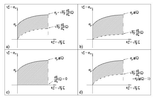
Fig. 3. Mechanical dissipation for the case of simple tension. The hatched area is the energy  $\int \Phi_m(t) dt$  dissipated during the monotonic loading. a) Classical Prandtl-Reuss model. b) Modified Prandtl-Reuss model. c) Modified Prandtl-Reuss model with  $\xi(\zeta) = \frac{d\xi}{d\zeta}(\zeta) = 0$ . d) Modified Prandtl-Reuss model with  $\sqrt{\frac{3}{2}} \frac{d\xi}{d\zeta}(\zeta) = \sigma_y(g(\zeta) - 1)$ : the classical model is recovered.
