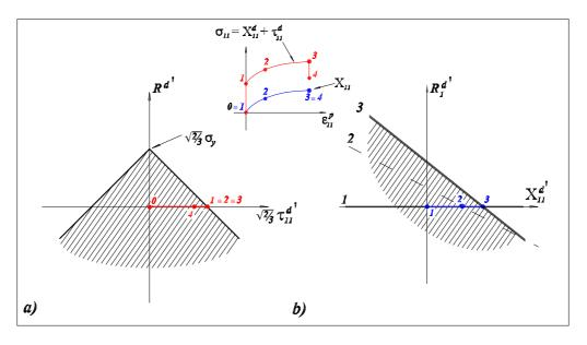
Fig. 8. NLK hardening model. Tension-compression case with  $g(\zeta)=1$ . a) Condition  $f\leq 0$  when  $R_1^{d'}=R_1^d=0$  and  $\mathbf{X}^{d'}=\mathbf{X}^d=\mathbf{D}:(\varepsilon^p-\beta)$ . b) Condition  $f\leq 0$  when  $R^{d'}=R^d=0$  and  $\|dev\left(\boldsymbol{\tau}^{d'}\right)\|=\|dev\left(\boldsymbol{\tau}^d\right)\|=\sqrt{\frac{2}{3}}\sigma_y$ .
