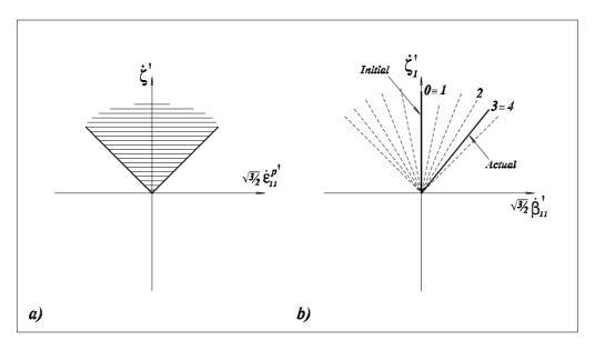
Fig. 7. NLK hardening model. Tension-compression case. a) Projection of the effective domain  $\bar{\mathbb{D}}$  on the  $(\dot{\varepsilon}^{p'}, \dot{\zeta}')$ -plane. b) Projection of  $\bar{\mathbb{D}}$  on the  $(\dot{\beta}', \dot{\zeta}'_1)$ -plane.
