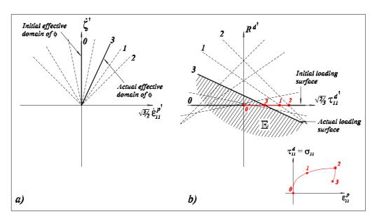
Fig. 4. Endochronic model. Tension-compression case with  $g(\zeta)=1$ . a) Several configurations of the set  $\mathbb{D}$ , which is the projection of the pseudo-potential effective domain  $\bar{\mathbb{D}}$  on the  $\left(\dot{\boldsymbol{\varepsilon}}^{p'},\dot{\zeta'}\right)$ -plane. b) Configurations of the convex set  $\mathbb{E}$  associated with those of  $\mathbb{D}$ . The point  $(\boldsymbol{\tau}^d,R^d)$ , representing the actual state, always lies on the axis  $R^{d'}=0$ .
