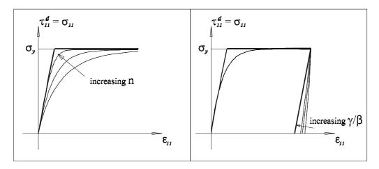
Fig. 5. Endochronic Karray-Bouc-Casciati model (thin lines) vs. Prandtl-Reuss model (thick line). Tension-compression case with  $g(\zeta)=1$  and  $\xi(\zeta)=0$ . a) Influence of the parameter n on loading branches. b) Influence of the  $\gamma/\beta$  ratio on unloading branches. The slope at  $\sigma_{11}=0$  is the same for all  $\gamma/\beta$  values.
