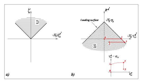
Fig. 1. Classical Prandtl-Reuss model. Tension-compression case. a) Projection of the pseudo-potential effective domain  $\bar{\mathbb{D}}$  on the  $\left(\dot{\varepsilon}^{p'},\dot{\zeta}'\right)$ -plane. This set is indicated by  $\mathbb{D}$ . b) Domain  $\mathbb{E}$  associated with the dual pseudo-potential  $\phi^*$ .
