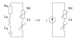
Fig. 2. Amplifier impedance determination
