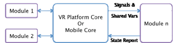
Fig. 5: The communication between the VR/Mobile core and the modules. The cores have the same architecture just modules are different.
