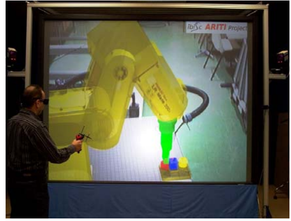
Fig. 2: The operator controls the virtual phantom robot to take virtual objects. After the validation, the distant real robot will follow the phantom and take the real objects
