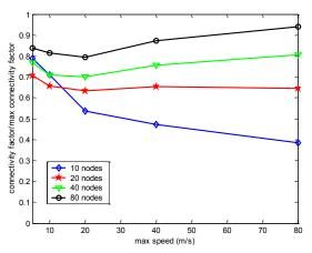
Fig. 6 Connectivity ratio vs max speed.
