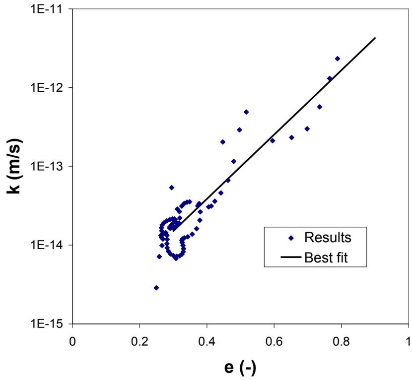
Figure 19. Test T04. Hydraulic conductivity versus void ratio.
