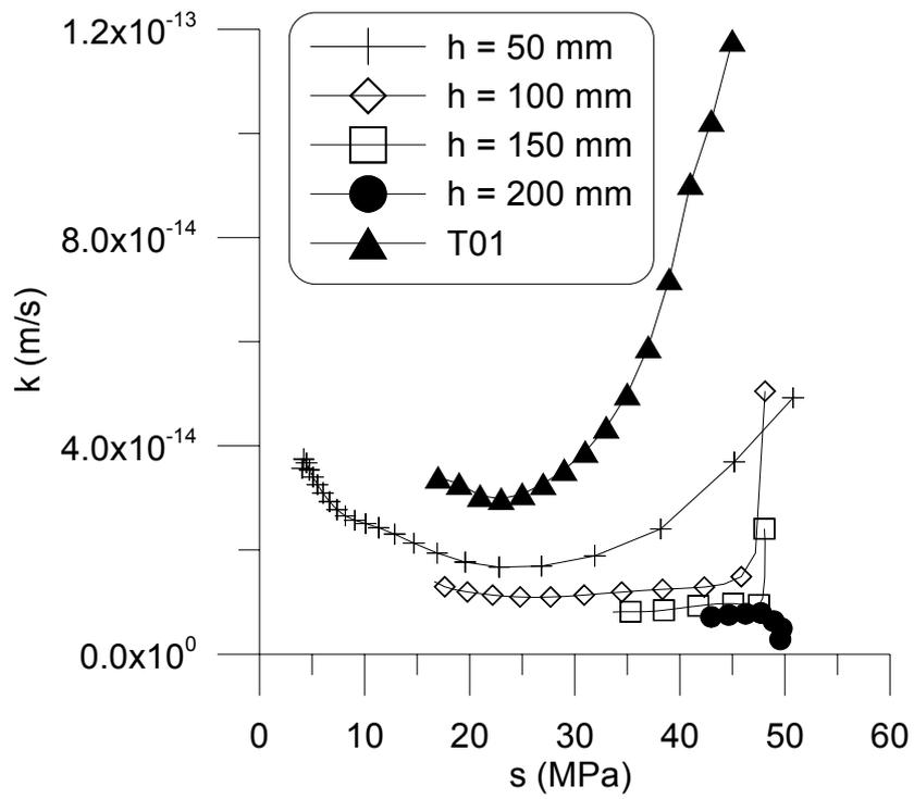
Figure 13. Test T01. Hydraulic conductivity versus suction.
