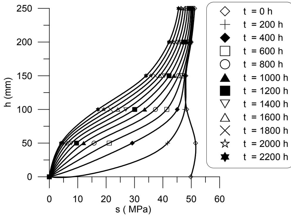
Figure 7. Test T01. Suction profile at different times.
