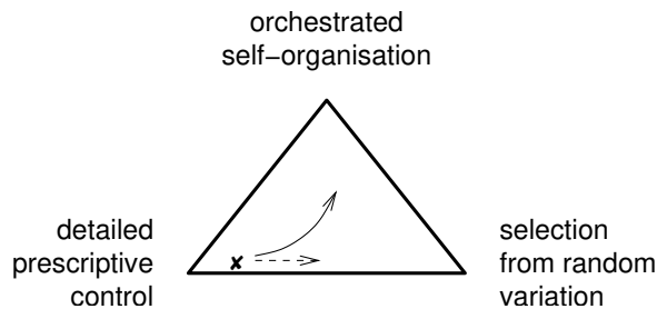
Fig. 2. Implementation paradigms for a computational device. Present conventional computer technology is indicated near the lower left corner. Random variation enters unintentionally in the production process. With increasing miniaturisation control will become increasingly more difficult (dashed arrow). Resilient architectures that can cope with wide component variation and the deliberate use of self-organisation processes provide the most likely path to complexification of computing architectures (bent arrow).
