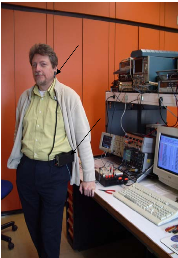
Fig. 4. Real-time and experimental wearable personal terminal for televigilance [10], equipped of sensors for heart rate (on ear) and actimetry (inside), with the in-door reception base-station: various physiological values on the blue display after fusion processing performed within the base-station.
