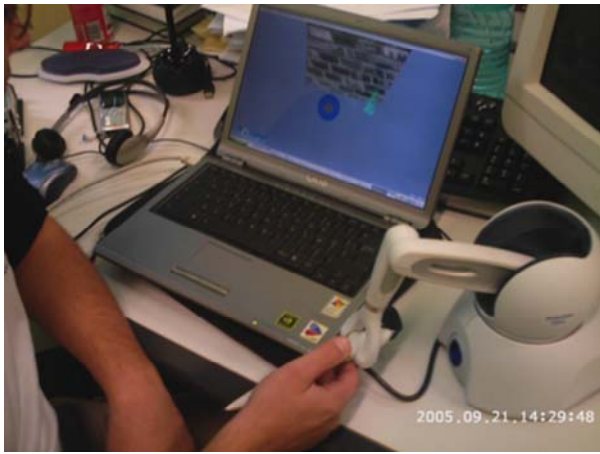
Fig. 9. Experimentation setup using an OMNI device and I-TOUCH Framework
