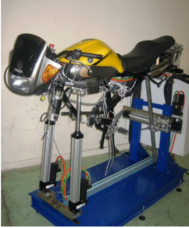
Fig. 6. Constructed riding motorcycle simulator
