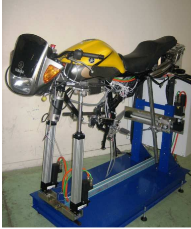
Fig. 6. Constructed riding motorcycle simulator
