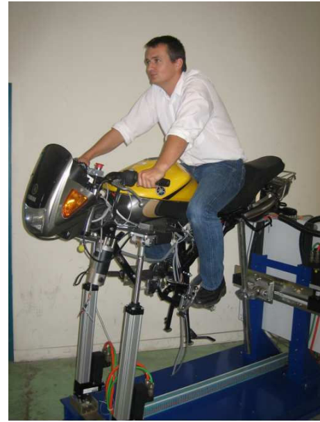
Fig. 6. Constructed riding motorcycle simulator
