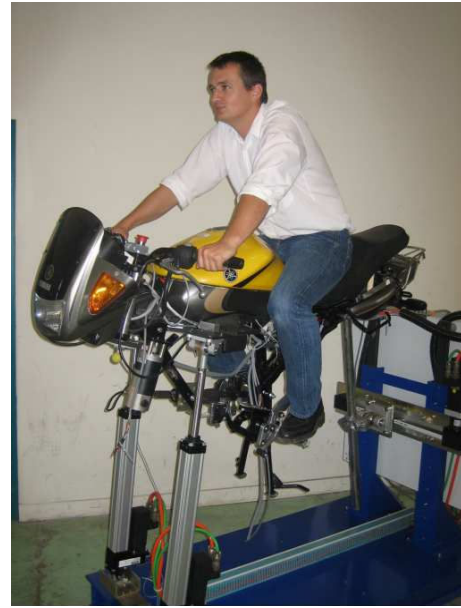
Fig. 6. Constructed riding motorcycle simulator
