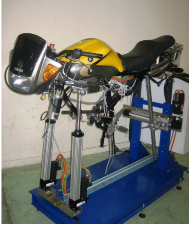
Fig. 8. Constructed riding motorcycle simulator
