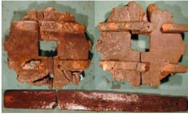
Figure 2: Photos of the fractured fountain parts.
