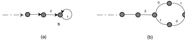
Fig. 6. Eliminating a self-loop
