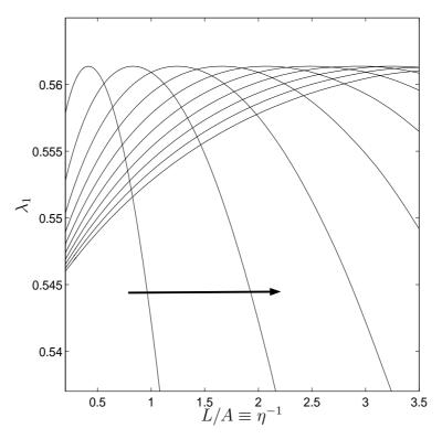
Figure 5: A plot of critical values of  $\lambda_1 \equiv \lambda(\rho_1)$  against undeformed length L/A for mode numbers  $n = 1 \div 10$  (see also Figure 5 in reference [11]). The arrow indicates the direction of increasing n.
