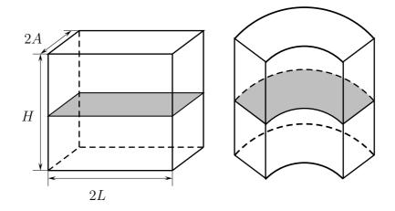
Figure 1: Cylindrical bending of a rubber block; left: *reference* configuration, right: *current* configuration. Shaded areas indicate two generic cross-sections perpendicular to the vertical axis.
