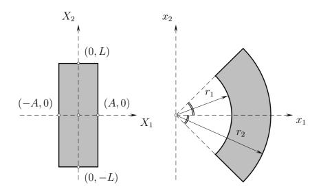
Figure 2: The undeformed (left) and deformed (right) cross-sections of the rubber block shown in Figure 1. Bending is symmetric with respect to the  $x_1$ -axis so that the two angles marked are congruent and equal to  $\omega_0$ ; see the text for more details.
