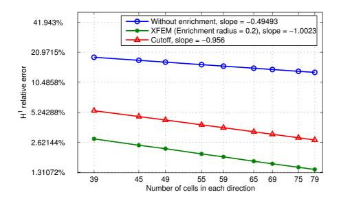
Figure 8:  $H^1$  error with respect to the number of cells in each direction (ns) for a mixed mode and different enrichment strategies of a P1 elements (from [12]).
