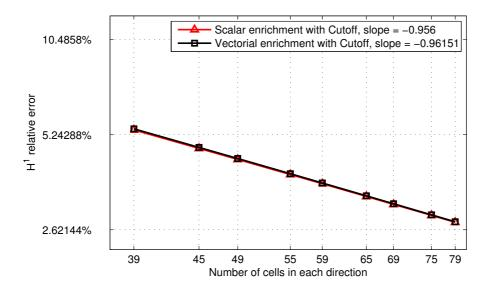
Figure 9:  $H^1$  error with respect to the number of cells in each direction (ns). Comparison of strategies (12) and (13).
