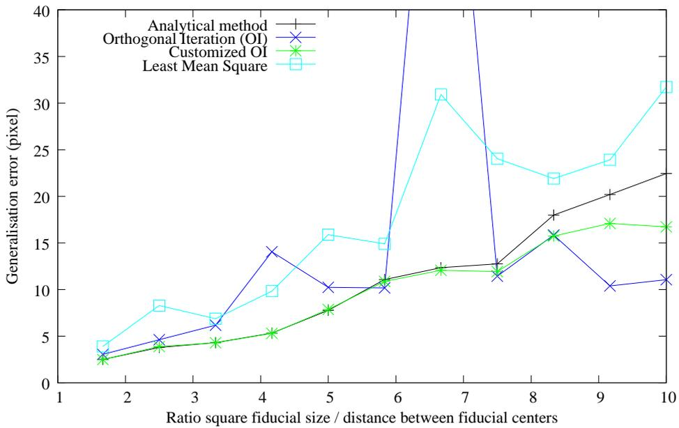
Fig. 6. Generalization error according to distance separating fiducials
