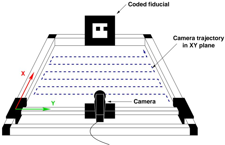
Fig. 8. Camera trajectory in the XY robot plane
