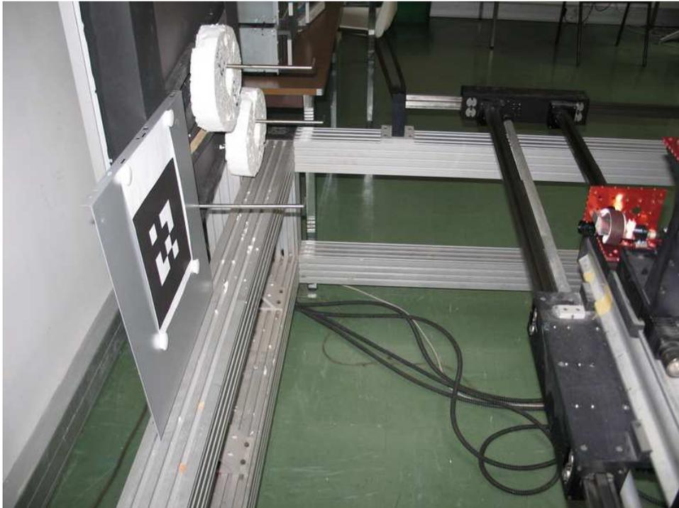
Fig. 7. Robot test-bench for distance estimation error
