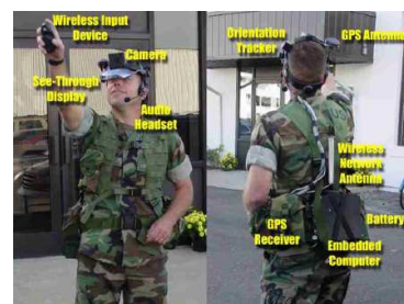
Figure 9: BARS platform [23] tested by a soldier
