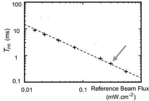
**Figure 12.**  $T_{PR}$  in  $ms$  as a function of the reference beam flux in  $W/cm^2$ . Crosses are experimental data. Dashed line is data extrapolation with slope  $-1$ . Grey arrow corresponds to Fig.7 experimental conditions.
