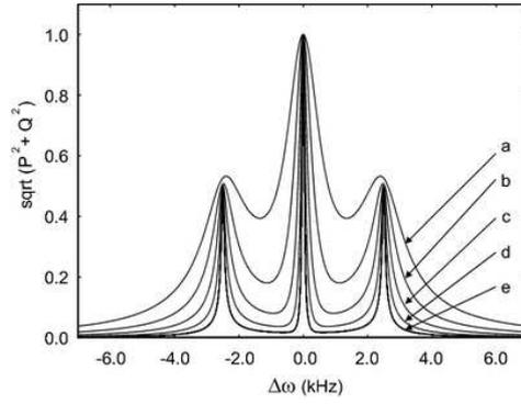
**Figure 10.** Calculated spectrum of the tagged photons signal (amplitude modulation with 50% cycling ratio) with  $T_{PR} = 0.25ms$  (a),  $0.5ms$ , (b),  $1ms$  (c),  $2ms$  (d),  $4ms$  (e). Horizontal axis is the frequency offset  $\Delta\omega$ . Vertical axis is  $\sqrt{P^2 + Q^2}$  lock-in signal in arbitrary normalized units.
