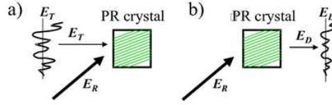
**Figure 3.** Principle of holography using the photorefractive effect.
