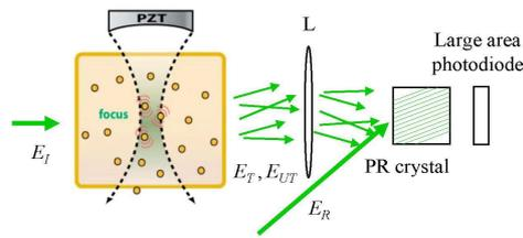
**Figure 2.** Principle of the PR detection of the acousto-optic signal. PZT: ultrasound transducer,  $E_I$ : illumination optical field;  $E_T, E_{UT}$  tagged or untagged field scattered by the sample; PR crystal: photorefractive crystal; L: lens that collect the scattered field into the crystal and photodiode;  $E_R$ : PR crystal reference (or pump) field.
