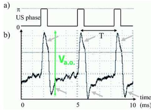
**Figure 7.** Typical tagged photons experimental signal. a) Modulation of the US phase
