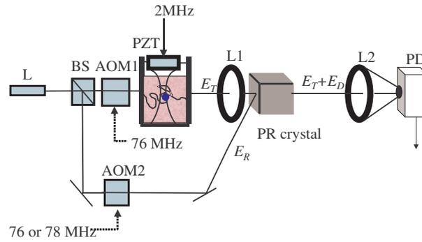
**Figure 6.** Typical experimental setup. L: laser; BS: Beam Splitter; AOM1, AOM2: acousto optic modulators; PZT: US generator; L1, L2: light collecting lenses; PR: photorefractive crystal; PD: photo detector.
