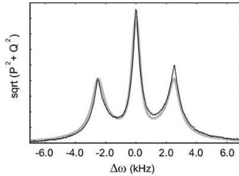
**Figure 11.** Spectrum of the tagged photons signal with 50% duty cycle amplitude modulation of the US. Black curve is experimental data with reference beam flux of  $300mW/cm^2$  and a modulation frequency of  $2.5kHz$ . Heavy grey line curve is calculated spectrum with  $T_{PR} = 0.45ms$ . Horizontal axis is the frequency offset  $\Delta\omega$ . Vertical axis is  $\sqrt{P^2 + Q^2}$  lock-in signal in arbitrary units.
