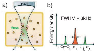
**Figure 1.** Principle of acousto-optic imaging. a) Motion of the scatterer at  $\omega_A$ . b) Spectrum of the diffused light: carrier ( $\omega_L$ ), and sideband i.e. tagged photons ( $\omega_L \pm \omega_A$ ).
